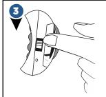
To turn on the invisible wall slide the switch away from the light towards the (I) symbol. Wait 10 seconds between turning it on or off.
