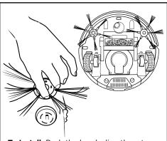
**To Install:** Push the brush directly onto the holder.
