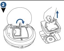
Pull up the dust bin handle and take out the dust bin from the robot.
