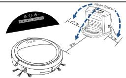
To test the auto-charge feature of the dock, turn the power switch ON and select "00" with the center button (see page 9 for control panel details). The vacuum should back into the dock for recharging if the appropriate spacing was provided for the docking station.
